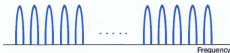
Figure. Frequency Division Multiplexing (FDM) Spacing is put between two adjacent sub-carriers.
