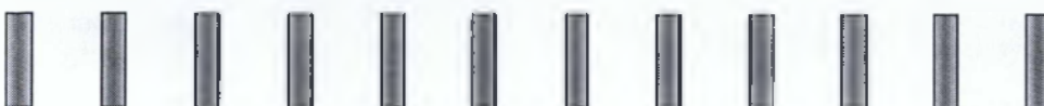
Transmitted upstream OFDM spectrum from the CPE using only a quarter of the carriers, but at the same level as the base station, hence the range will be the same with a quarter of the capacity
