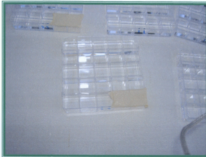
Picture 10 Plastic tray covered with tape in the control leaf positions
