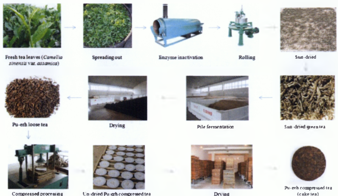
Fig. 2. Flow diagram of the modern manufacture process of Pu-erh tea.
